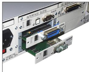
Programming via a data interface extends the functional range of the ZSAC Load by many dynamic functions in connection with synchronous measurement storage. The interface cards are pluggable and can be exchanged or extended as required.
