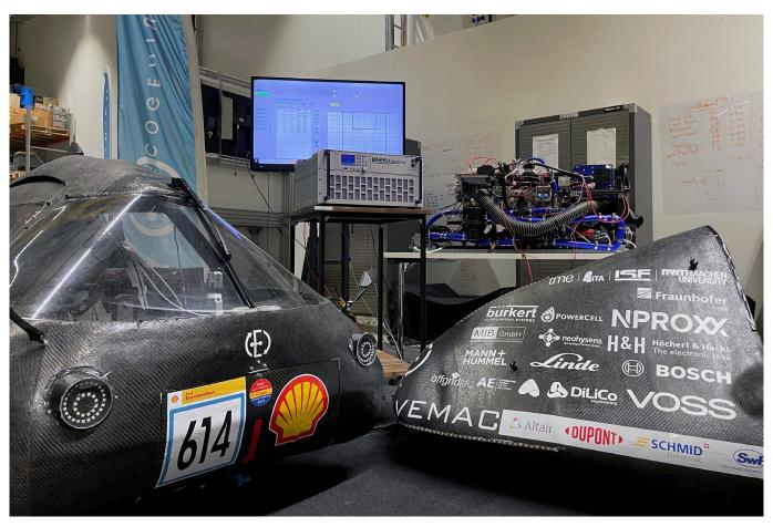
The vehicle requires different voltage levels; for example, the control unit is operated at 12 V, while the engine controllers are operated at 53 V. To be able to supply all devices with the fuel cell, DC/DC converters are used. The PLI4806 is also used for load testing and efficiency determination of the DC/DC converters. With its input voltage range up to 60 V, all necessary voltages are covered.
