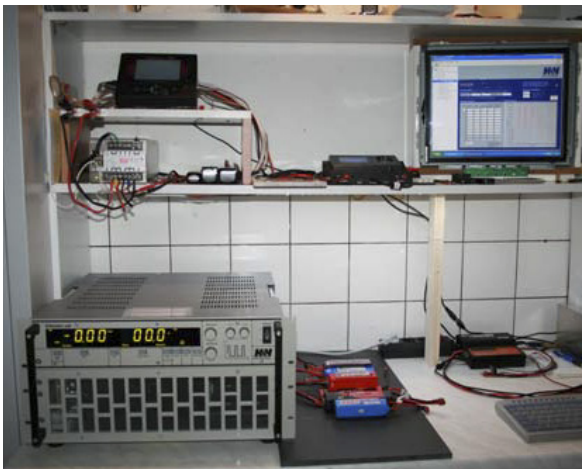
The ZS3006 from Hoecherl & Hackl already found its place in the author's workshop. However, a proper operation without a PC does not make much sense because the PC is required to create the load profiles as well as to analyze the measured data and the graphical preparation of the measurement records.
