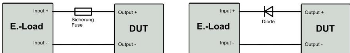
Figure 2.27: Reverse voltage protection by fuse (left) or diode (right)
