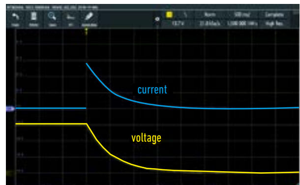
Discharging: C = 1\text{ F} without R_i , using an external charging resistor R = 0.56\ \Omega .
